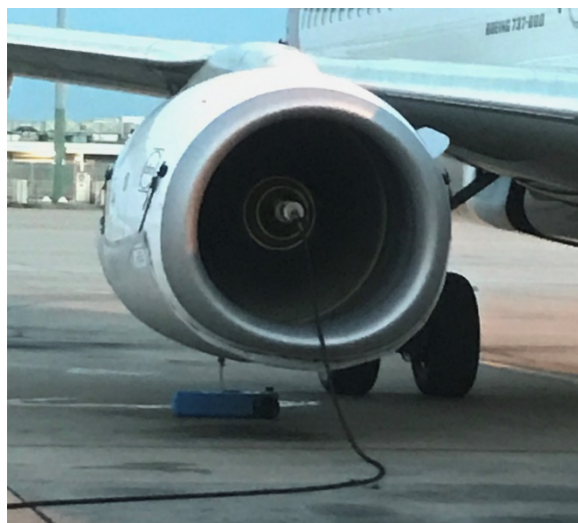
A new compressor wash system with detergent recovery.
